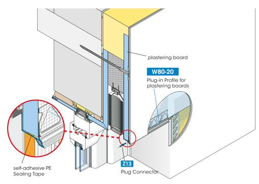
The plastic APU Plug-in Profile W80 for plastering boards with thickness of 10, 12, 15 and 20 mm is used for shutters/lamellar blind boxes as plaster border profile.
