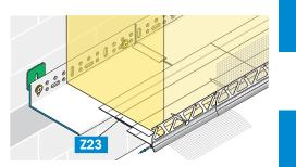
**Example** with 2 Extensions for an insulation thickness of 300 mm
