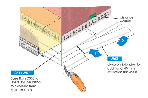
Cut the plastic Base Rail Extension W63 with Trimming Shears or suitable tools and clasp it onto the finished mounted Base Rail (first clip on one end, then press the Extension towards the other end into position - see illustration - for easier working). Set the extensions always offset to the contact area between two Base Rails.
