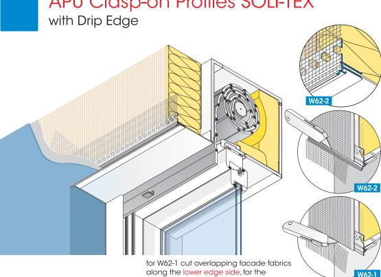
Plaster borders in thermal insulation composite systems also require a secure solution with regard to water-guiding and drainage downwards.
