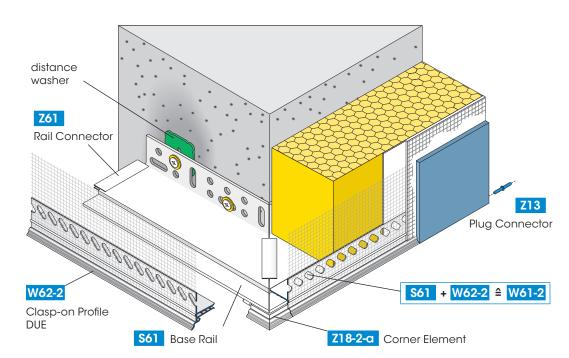
The Base Rails are made of plastic with a stepped bending for taking up a Clasp-on Profile with fabric and Drip Edge (fabric width 12.5 cm). It is suitable for insulation thicknesses of 50-200 mm in thermal insulation composite systems with rigid foam/mineral fiber boards and fabric filler of 4–8 mm. For improved adhesion of the plasters the transition to the Drip Edge is grooved.
