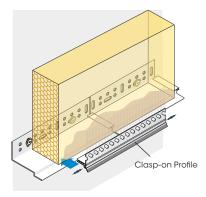
The Clasp-on Profiles W62 are slid in below the insulation board onto the stepped bending and aligned in a flush direction into the fixing mortar with Plug Connectors Z13 between two profiles. The Clasp-on profiles should alsways be installed overlapping the Base Rail joints for stabilization.
