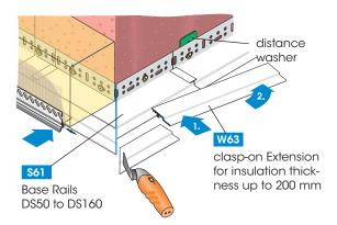
Cut the Extension W63 in the same way and clip it onto the finished mounted Base Rail S61 (first clip on one end, then press the Extension towards the other end into position - see illustration - for easier working).
