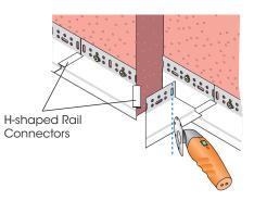
Cut the corner parts of Base Rails in place using a Multimaster tool (type FEIN).
