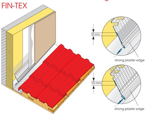
This pofile is slipped over sheet metal joints (e.g. roof borders) resulting into a movable water-proof joint between the plaster and sheet metal due to its hollow chamber. The sheet metal's equalization movements are buffered by the profile which prevents cracks in the plaster. The finished plaster edge (W45-8 for 8 mm plaster thickness and W45-11 for 11 mm plaster thickness) ensures a well-directed water guiding.
