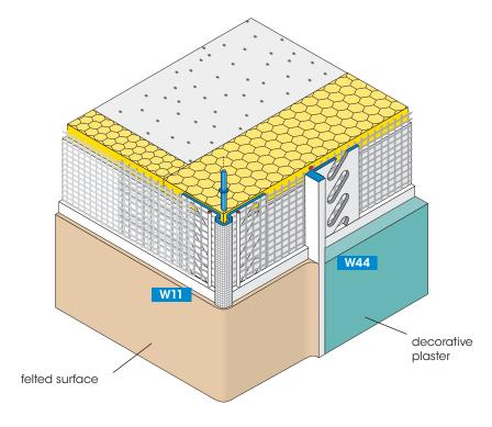
The Border Profile with welded on fabric part forms plaster edges in the final plaster of thermal insulation composite systems.
