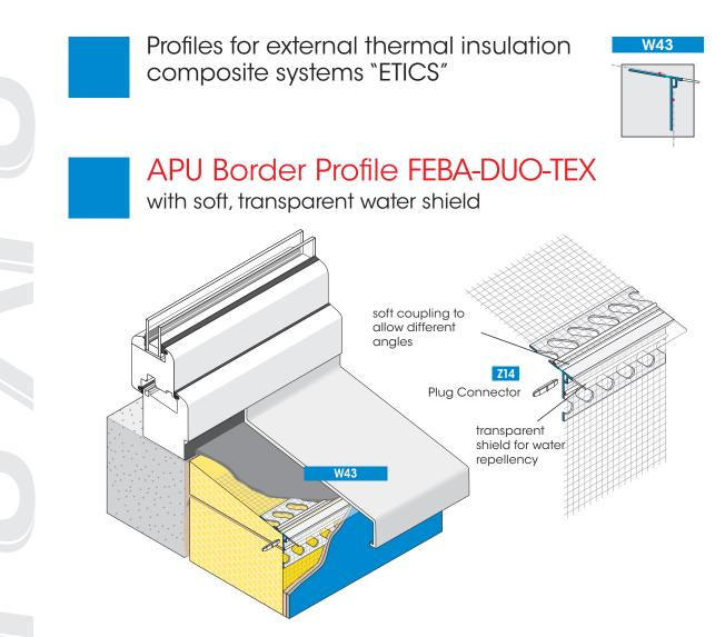
The border profile FEBA-DUO-TEX forms in combination with a second sealing level a clean plaster finish under the window sill.
