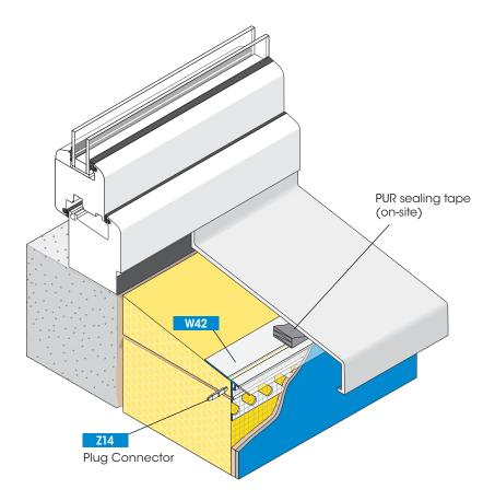
Even without a second sealing level the border profile FEBA-TEX-UNI forms a clean plaster finish under the window sill.
