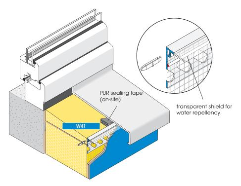
The border profile FEBA-TEX-ATTIKA forms a clean plaster finish under the window sill, in Attic regions behind sheet metal cladding or similar applications.
