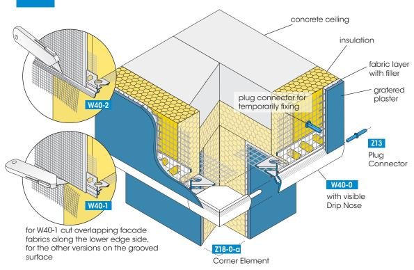
Plaster borders in thermal insulation composite systems also require a secure solution with regard to water-guiding and drainage downwards.
