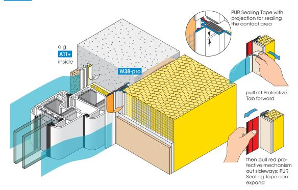
The APU Joint Profile with fabric PUR-FIX-pro is used in ETIC systems and window and door systems where bigger equalization movements are expected. The profile can be aligned and set before the insulation is applied.
