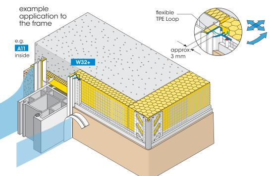
The Joint Profile with fabric MILANO-plus is intended for ETIC systems with deep insulation reveals, insulation thicknesses up to 160 mm and windows aligned with the masonry.
