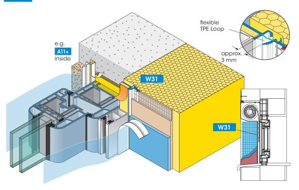
Projecting roller shutter systems are constructed to avoid cold bridges. The inspection flaps are located exterior and the plaster joint is made laterally to the guide rails.
