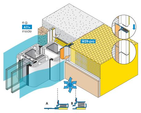
Factory-provided PUR Sealing Tape projection to seal the contact area between the profiles
