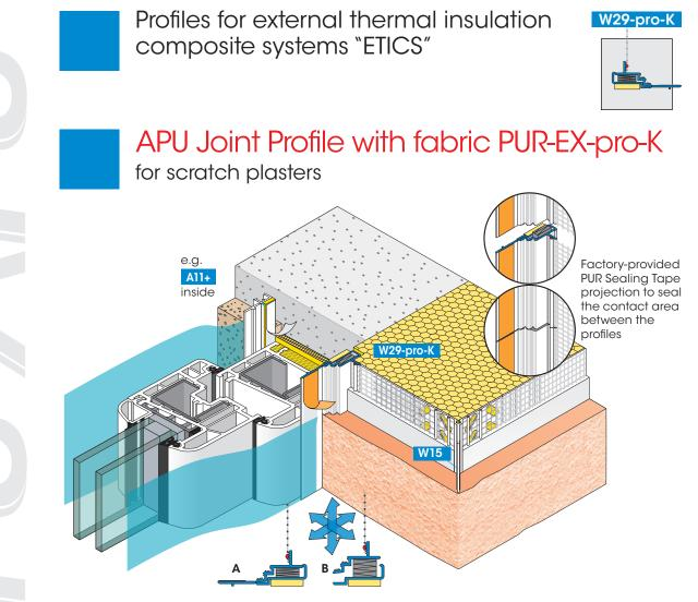
The APU Joint Profile with fabric PUR-EX-pro-K is equipped with a compressed and pushed in PUR Sealing Tape (A), which is released by removing the Protective Tab, and expands freely as required (B). It provides a decoupled (\*) solution between a plaster system and the framework.
