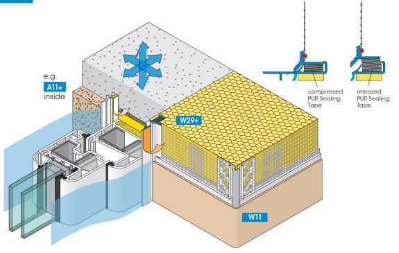
The APU Joint Profile with fabric PUR-EX (and PUR-EX-plus - with a soft Protective Lip) is equipped with a compressed and pushed in PUR Sealing Tape which is released by removing the Protective Tab, and expands freely as required. It provides a decoupled (\*) solution between plaster system and the framework.
