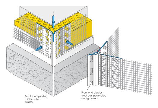
The Corner Bracket with fabric STABILO is provided with wide plastic flanks with two rows of perforations. The fabric parts fastened each with two welding cords that form the plaster level bars for the filler layer high.
