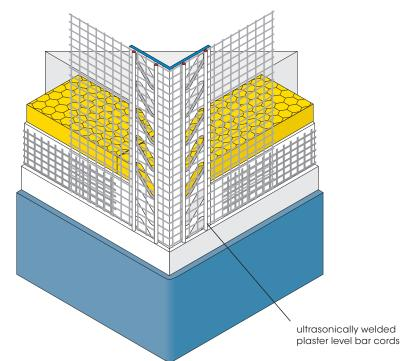
A new generation Corner Bracket made of plastic, with large elongated perforations facilitating convenient passage for coating material.
