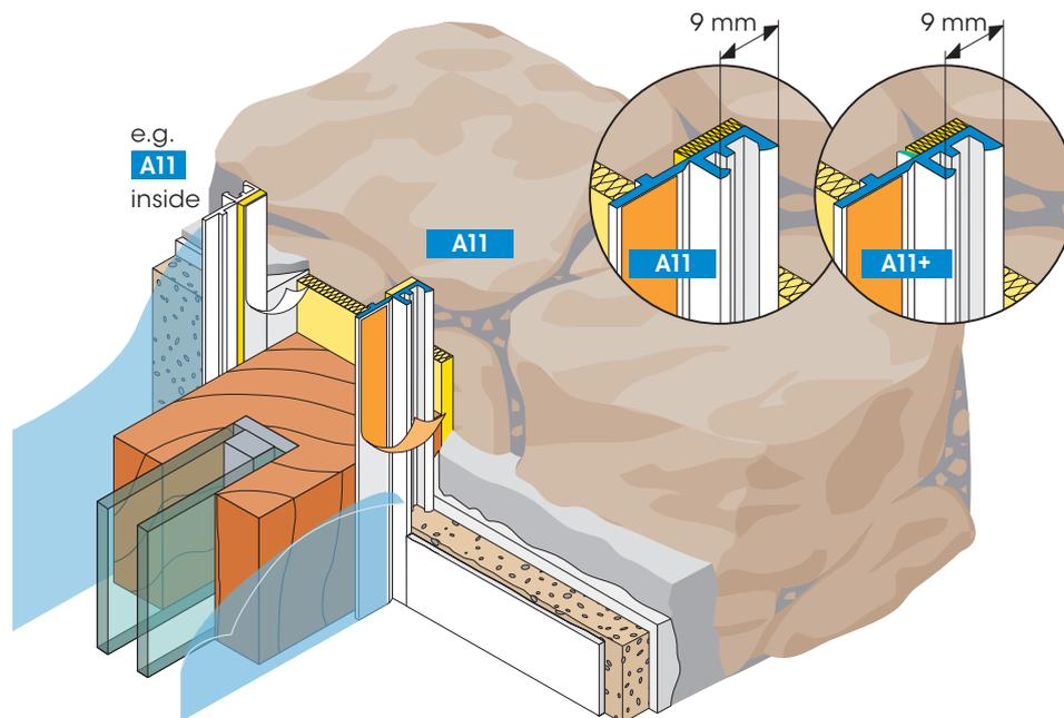
Reworked plaster surfaces and internal plasters require compact and secured plaster joints to doors, windows and other component parts.
