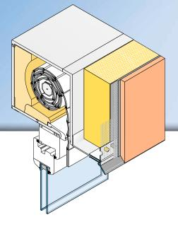
The **APU clip-on profile QUATTRO** is used horizontally in compound heat insulation systems e.g., for plaster joints up against shutter boxes or in the base area.
