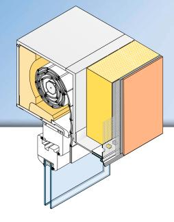
The **APU clip-on profile DUE** is used horizontally in compound heat insulation systems e.g., for plaster joints up against shutter boxes or in the base area. The cranked profile contour provides a reliable solution in respect of downward guidance of water.
