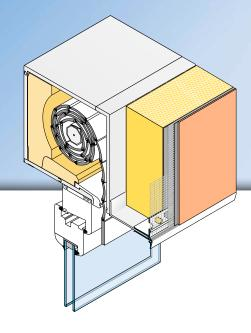
The **APU clip-on profile ZERO** is used horizontally in compound heat insulation systems e.g., for plaster joints up against shutter boxes or in the base area. The profile contour with visible drip edge provides a reliable solution in respect of downward guidance of water.
