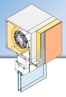
The **APU stick-on profile UNO** is used horizontally in compound heat insulation systems e.g., for plaster joints up against shutter boxes.
