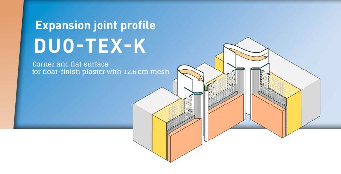
The **APU expansion joint profile DUO-TEX-K** is used in compound heat insulation systems at building joints.
