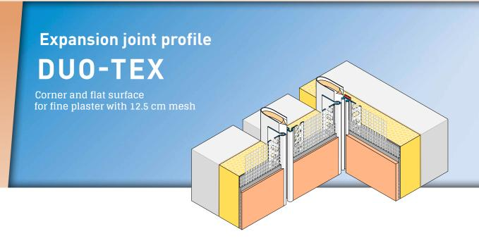
The **APU expansion joint profile DUO-TEX** is used in compound heat insulation systems at building joints. For the flush formation of a clean plaster edge, the profiles for surface areas (W52) and for inner corners (W51) are made.
