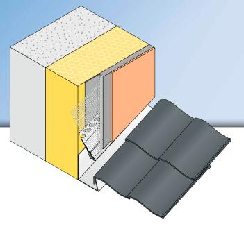
The **APU flashing bead PUR-FIX** is used at junction points with metal plate in compound heat insulation systems (e.g., at junctions with the roof's edge) and as a result of its integrated PUR sealing strip produces a flexible connection between plaster and metal. When the plaster work is finished, the profile ensures that water is accurately guided away.
