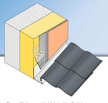
The APU flashing bead FIN-TEX MINI is used at junction points with metal plate in compound heat insulation systems (e.g., at junctions with the roof's edge) and as a result of its cavity design produces a flexible connection between plaster and metal. The profile is used for 8 mm plaster thickness and upon completion of the plastering work ensures that water is accurately guided away.
