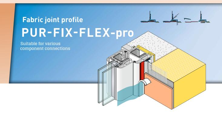
The APU fabric joint profile PUR-FIX-FLEX-pro is used in compound heat insulation systems as specified in the latest APU selection criteria. By virtue of its flexible characteristics on the fixation flank and plaster bar it can also be used, for example, for recesses with a lighting wedge, for GFB base elements and in many other installation situations. What is created after completion of the plastering work is a clean and safe termination of the plaster with shadow gap.
