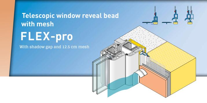
The **APU telescopic window reveal bead with mesh FLEX-plus** is used in compound heat insulation systems as specified in the latest APU selection criteria.
