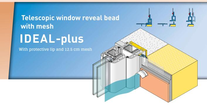
The APU telescopic window reveal bead with mesh IDEAL-plus is used in compound heat insulation systems as specified in the latest APU selection criteria. In front of the reveal insulation the profile is stuck flush to the structural element there and after completion of the plastering work forms a clean and reliable termination of the plaster.
