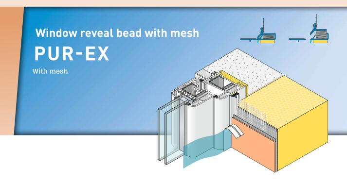
The APU window reveal bead with mesh PUR-EX is used in compound heat insulation systems as specified in the latest APU selection criteria. Within the reveal the profile is stuck flush to the structural element there and thus forms a clean and reliable termination of the plaster.
