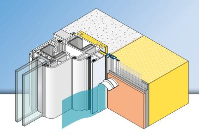
The APU telescopic window reveal bead IDEAL-R is used in external thermal insulation composite systems (ETICS) in accordance with the current APU
