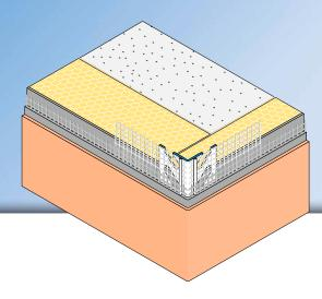
The **APU corner bead with mesh ULTRA-TEX** is used in compound heat insulation systems as a flush, impact-protected edge for thin top layers of plaster.
