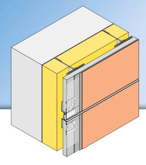
For back-ventilated rainscreens the **APU joint profile VHF-PRO-TEX** is used as a termination onto the edge of the supporting board. In combination with the VHF-DROP-TEX (V82) joint profile the area boundary joint is thus formed horizontally and vertically and a clean plaster edge with shadow gap is created.
