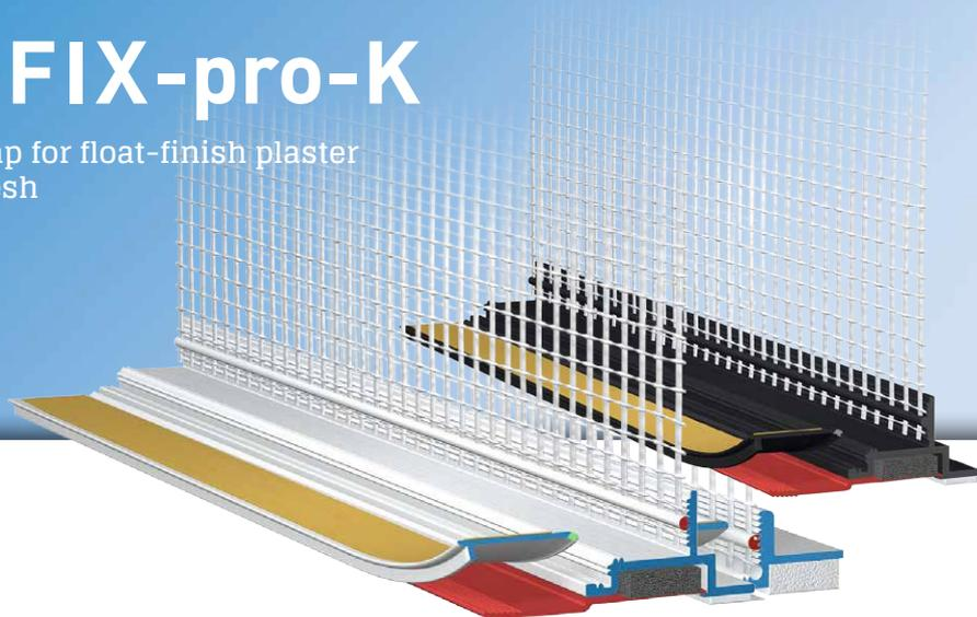
The **APU window reveal bead with mesh PUR-FIX-pro-K** is used in compound heat insulation systems as specified in the latest APU selection criteria. The profile is put in place shortly before the insulation of the reveal, is fixed flush to the structural element and after completion of the plastering work provides a clean and reliable termination of the plaster with a shadow gap. The profile contour enables the application of a thick layer of plaster / float-finish plaster.
