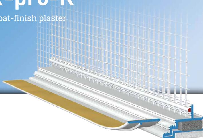
The **APU window reveal bead with mesh PUR-EX-pro-K** is used in compound heat insulation systems as specified in the latest APU selection criteria. Within the reveal the profile is stuck to the structural element there and thus forms a clean and reliable termination of the plaster with shadow gap. The profile contour enables the application of a thick layer of plaster / float-finish plaster.
