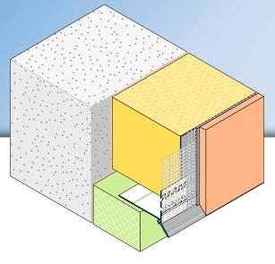
The APU base edge profile SOKA-TEX-QUATTRO is used in compound heat insulation systems as the bottom termination of the wall insulation.
