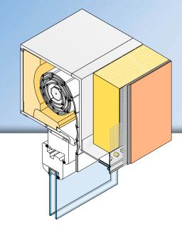
The **APU clip-on profile UNO** is used horizontally in compound heat insulation systems e.g., for plaster joints up against shutter boxes or in the base area. The straight profile contour provides a reliable solution in respect of downward guidance of water.
