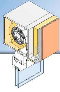
The **APU stick-on profile DUE** is used horizontally in compound heat insulation systems e.g., for plaster joints up against shutter boxes.
