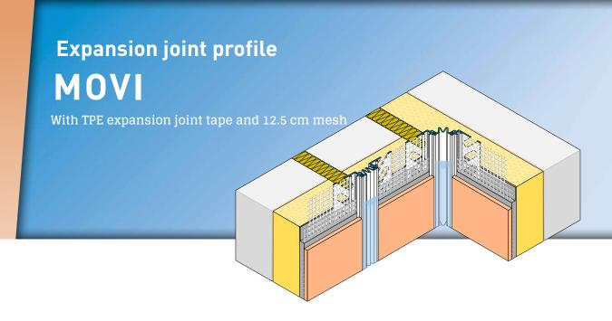
The **APU expansion joint profile MOVI** is used in compound heat insulation systems at vertical building joints. For the flush formation of a clean plaster edge, the profile can fitted both in flat surfaces and inner corners.
