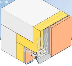
The **APU drip bead DROP-TEX-QUATTRO** is used horizontally in compound heat insulation systems for recessed building elements, such as window and door jambs.
