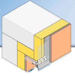
The **APU drip bead DROP-TEX-TRE** is used horizontally in compound heat insulation systems for recessed building elements, such as window and door jambs.
