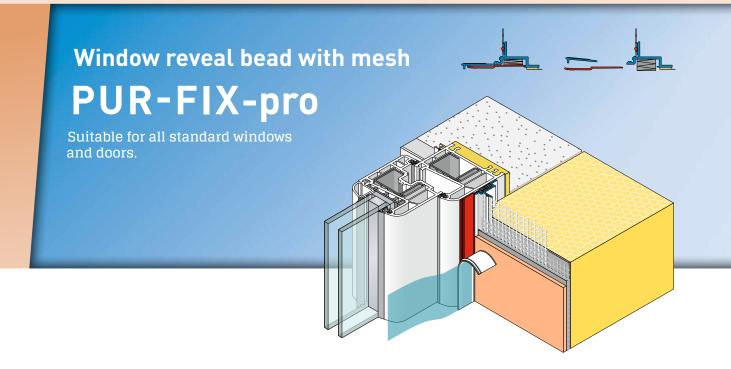
The **APU window reveal bead with mesh PUR-FIXpro** is used in compound heat insulation systems as specified in the latest APU selection criteria. The profile is put in place shortly before the insulation of the reveal, is fixed flush to the structural element and after completion of the plastering work provides a clean and reliable termination of the plaster with a shadow gap.
