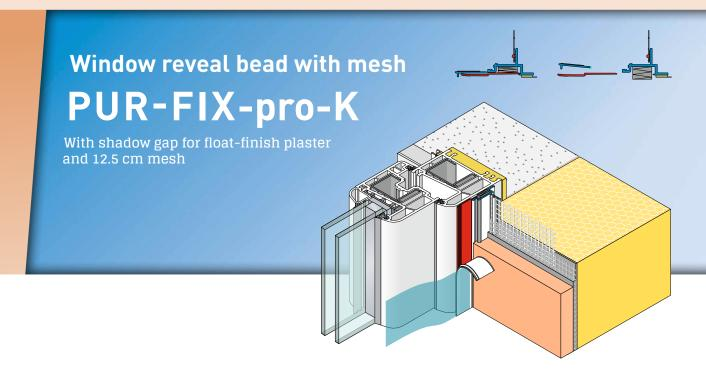
The APU window reveal bead with mesh PUR-FIX-pro-K is used in compound heat insulation systems as specified in the latest APU selection criteria. The profile is put in place shortly before the insulation of the reveal, is fixed flush to the structural element and after completion of the plastering work provides a clean and reliable termination of the plaster with a shadow gap. The profile contour enables the application of a thick layer of plaster / float-finish plaster.
