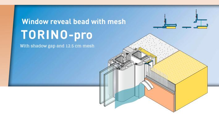
The APU window reveal bead with mesh TO-RINO-pro is used in compound heat insulation systems as specified in the latest APU selection criteria. Within the reveal the profile is stuck flush to the structural element there and after completion of the plastering work forms a clean and reliable termination of the plaster with shadow gap.
