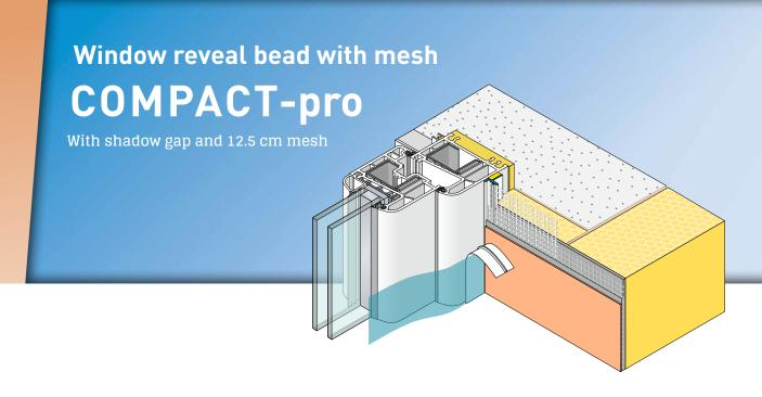
The APU window reveal bead with mesh COM-PACT-plus is used in compound heat insulation systems in accordance with the APU area of application. Within the reveal the profile is stuck flush to the structural element there and thus forms a clean and reliable termination of the plaster with shadow gap.
