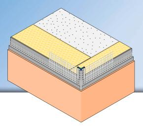
The **APU corner bead with mesh MINI** is used in compound heat insulation systems as a flush, impact-protected edge for thin top layers of plaster. If necessary, the bracket can be bent and thus made suitable for curves.
