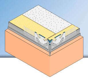
The **APU** corner bead with mesh **STABILO** is used in compound heat insulation systems as a flush, impact-protected edge for float-finish plaster and thick plaster layers.
