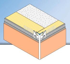
The **APU** corner bead with mesh DECO-TEX is used in compound heat insulation systems as a flush, impact-protected edge for thin top layers of plaster.
